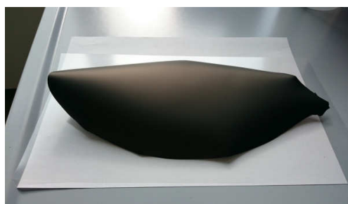
Figure 8. Green tape obtained by using powder D from slurry 5 (+33% plasticizer I) after drying.
